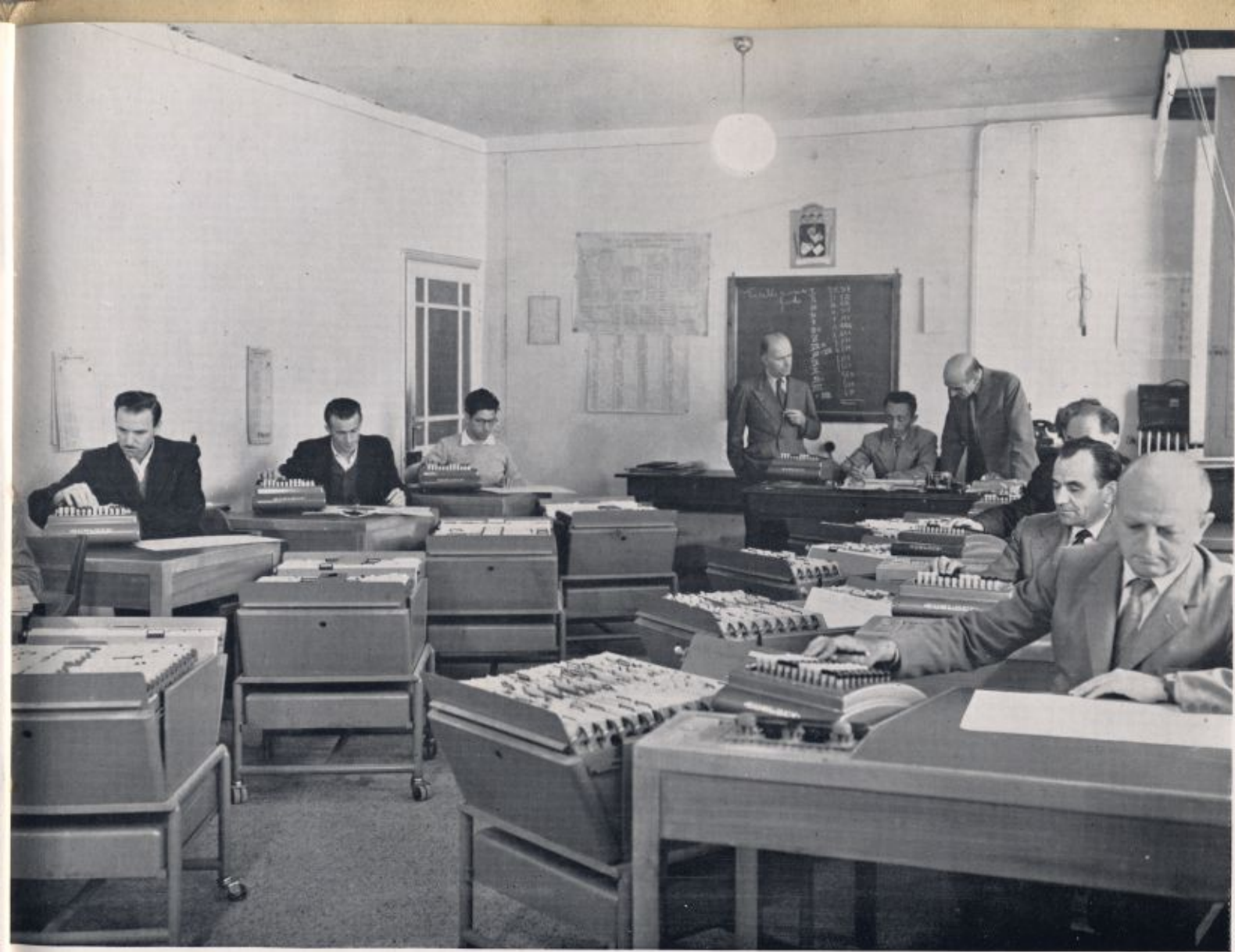
"Sumlocks" in use at the Administration Office of the Italian State Railways in Florence.
